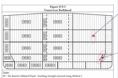
$\ensuremath{\mathrm{UP}}$  –  $\ensuremath{\mathrm{M2}}$  denotes Un-stiffened Panel – buckling strength assessed using Method 2
