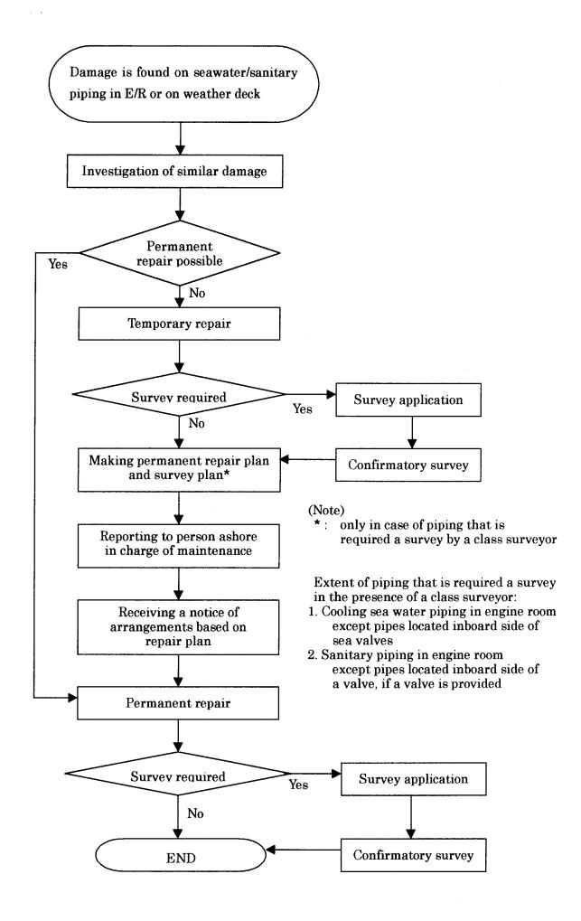
Flowchart for repair of piping in Engine Room and on weather deck
