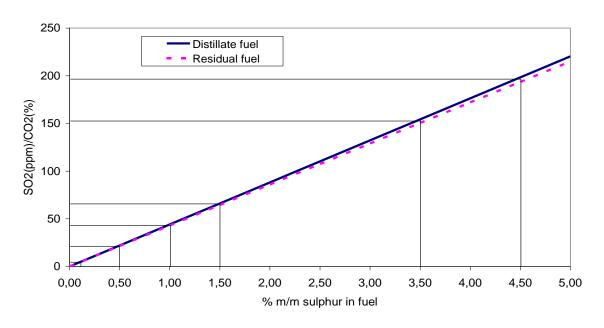
4 Correspondence between 65 (ppm<sup>4</sup>/%) SO<sub>2</sub>/CO<sub>2</sub> and 6.0 g/kWh is demonstrated by showing that their S/C ratios are similar. This requires the additional assumption of a brake-specified fuel consumption value of 200 g/kWh. This is an appropriate average for marine diesel engines. The calculation is as follows:
