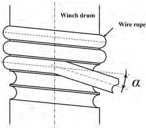
Fig. 7.2.2-2 Fleet angle of drum other than grooved drum
