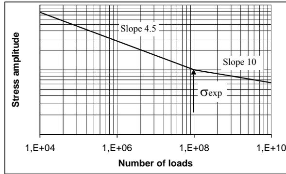
Fig. I58.9 Constant-slope S-N Curve
