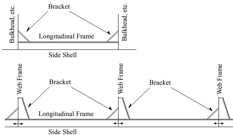
Fig. 158.3.2-2 Brackets for Transverse Side Frames
