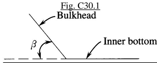
**3** In ships whose cargoes are regularly handled by grabs or similar mechanical appliances, the thickness of the longitudinal bulkhead plating is not to be less than the value obtained from the requirements in -2 above plus the following values. The extent of application of this requirement is to be as deemed appropriate by the Society.
