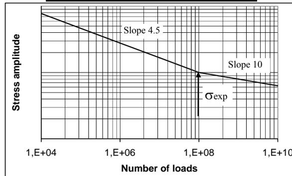
**Fig.I5.9 Constant-slope S-N curve**
