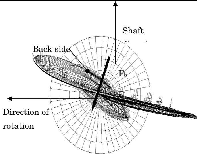
**2** The maximum backward blade force  $F_b$  is to be applied as a uniform pressure distribution to an area of the blade for the following load cases:
