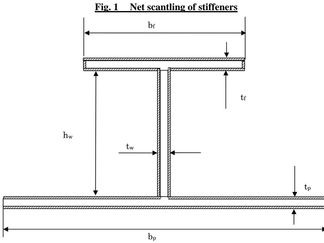
Shadow area is corrosion addition.
