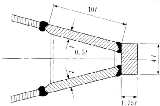
$t$  = Thickness (mm) of side plating
