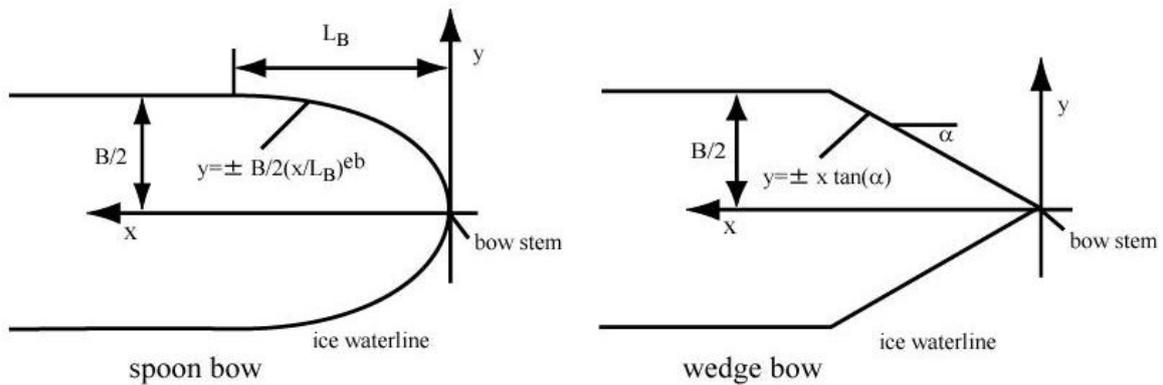
**Fig. I3.6 Illustration of  $e_b$  Effect on the Bow Shape for  $B=20$  and  $L_B=16$**
