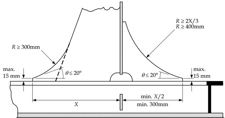
Recommended Design of Soft Toes and Backing Bracket of Tripping Brackets
