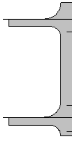
Fig. 8 Example of Insertion of Transverse Rib
