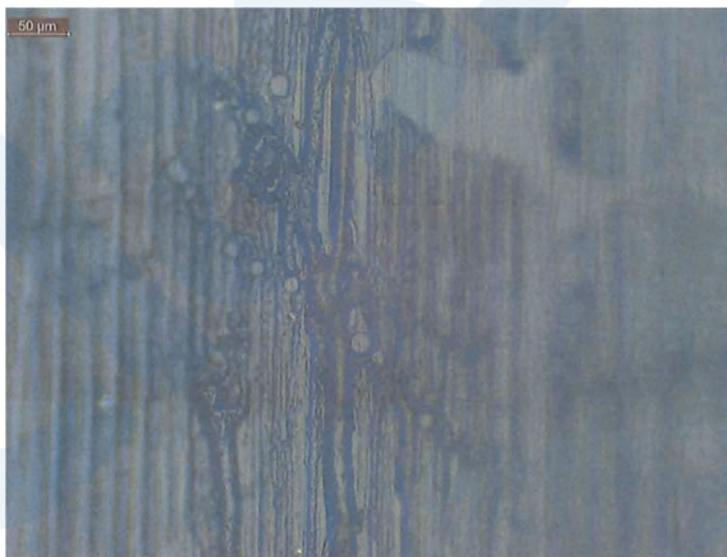
Figure 4 Cat-fines embedded in the cylinder liner and trace of abrasive wear
