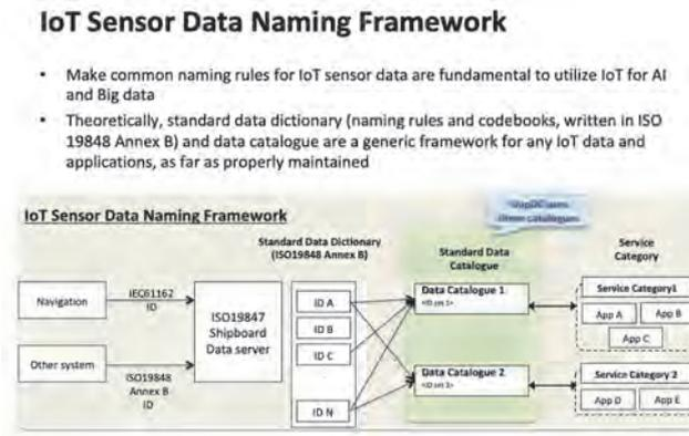
Fig.3 IoT Sensor Data Naming Framework
