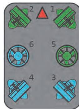
Figure 2 Motor Position and Facing direction
