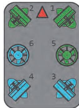
Figure 2 Motor Position and Facing direction
