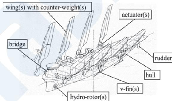
Figure 9 Basic arrangement of type C
