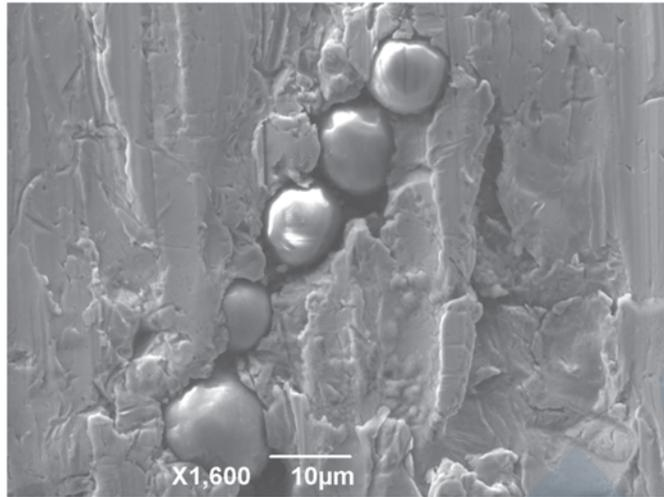
Figure 5 Cat-fines embedded in the piston ring
