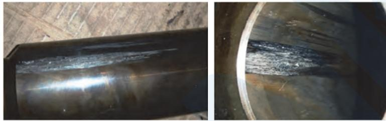
Figure 3 Scratches on the plunger and barrel in the fuel injection pump
