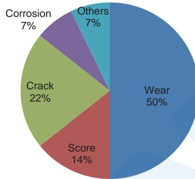
Fig. 17 Breakdown of type of damage for cylinder liner
