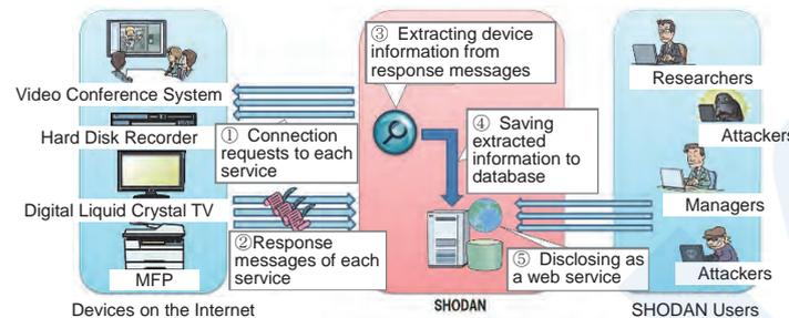
Fig. 4 Mechanism of SHODAN
