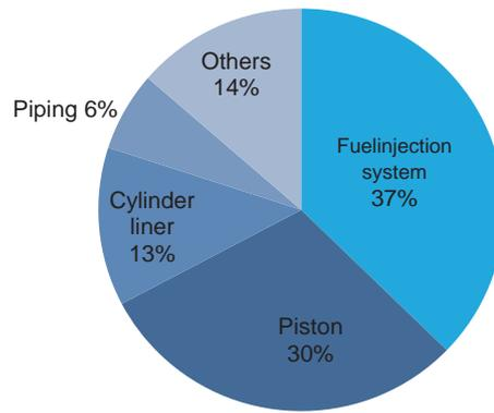
Fig. 9 Breakdown of damaged components of diesel engines
