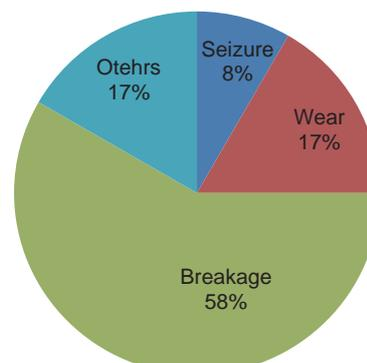
Fig. 16 Breakdown of type of damage for piston ring
