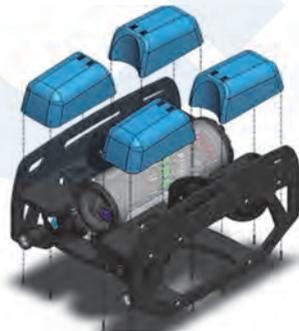
Figure 1 Position of the Enclosures and Buoyancy
