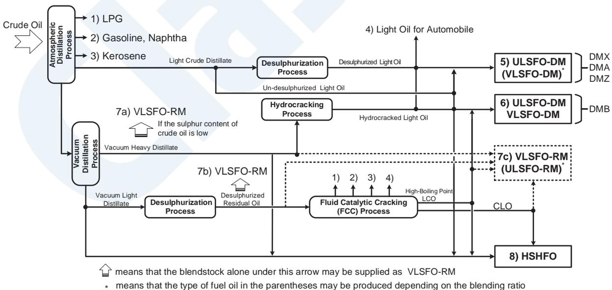
Figure 1 The possible blending process to produce marine fuel oils<sup>4)</sup>
