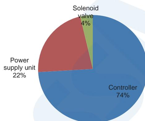
Fig. 6 Breakdown of damaged parts in the electrical and control systems
