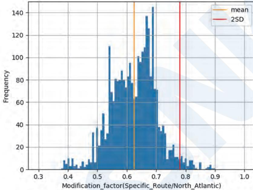
Figure 9 Histogram of modification factors of loads for feeder container carriers
