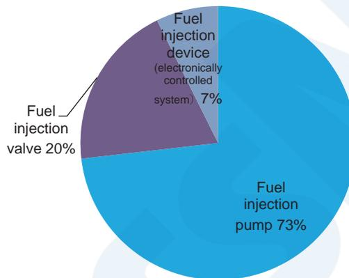
Fig. 10 Breakdown of damaged parts of the fuel injection system in diesel engines
