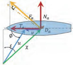
Figure 3 Composition of the propulsive Force
