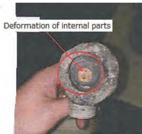
Photo 3 Fresh-water level switch with deformed internal part
