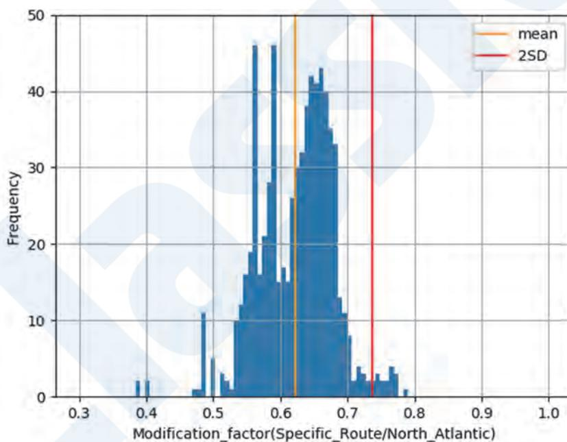
Figure 6 Histogram of load modification factors for VLCCs
