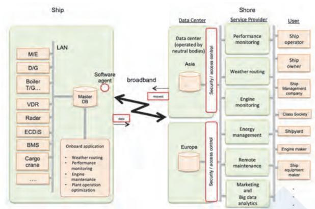
Figure 2 Conceptual Diagram of the Open Platform between Shore and Ship
