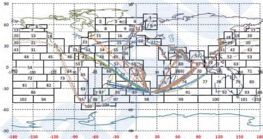
Figure 8 Operating routes of the top 14 VLCCs whose load modification factors are less than or equal to the mean value plus twice the standard deviation
