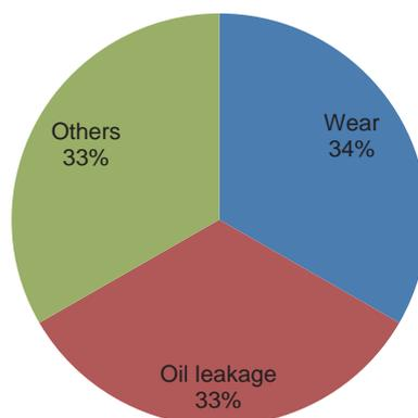
Fig. 13 Breakdown of type of damage for fuel injection device (electronically controlled system)
