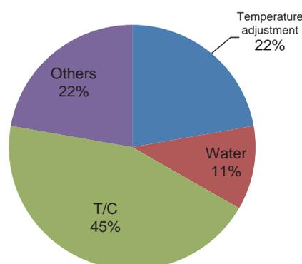
Fig. 19 Breakdown of secondary damage due to fuel oil and malfunction due to improper handling of fuel oil
