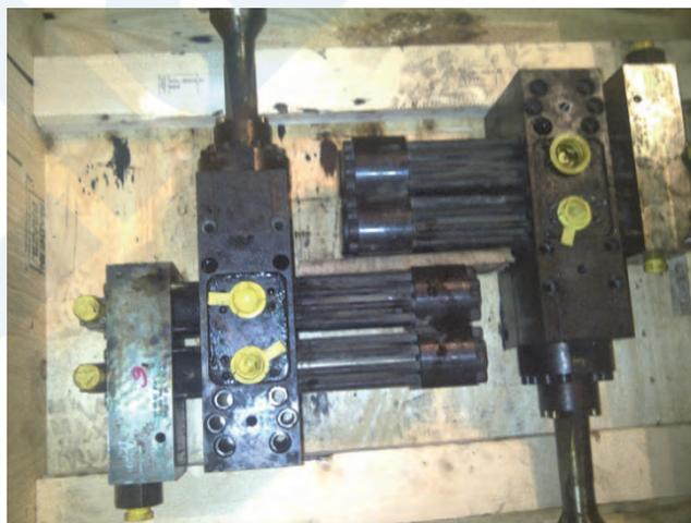
Photo 5 Fuel injection control device from which fuel oil leaked
