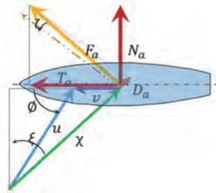
Figure 3 Composition of the propulsive Force
