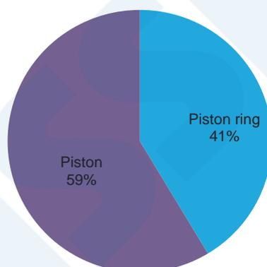
Fig. 14 Breakdown of damaged parts of piston
