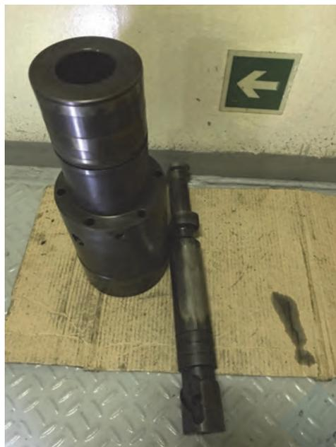
Photo 4 Seizure of plunger and barrel
