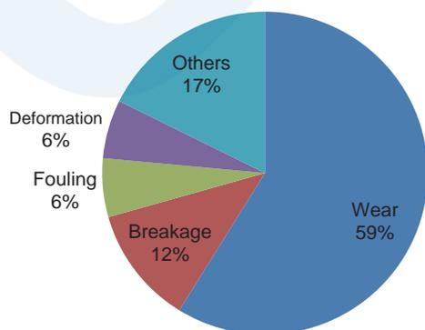
Fig. 15 Breakdown of type of damage for piston
