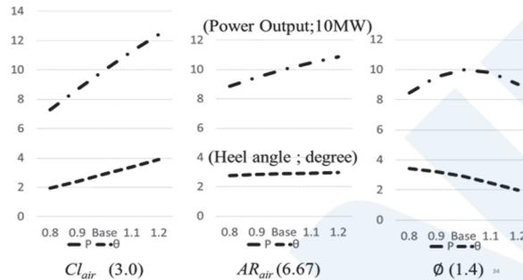
Figure 10 Sensitivity according to the aerodynamic property
