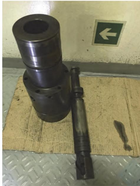
Photo 4 Seizure of plunger and barrel
