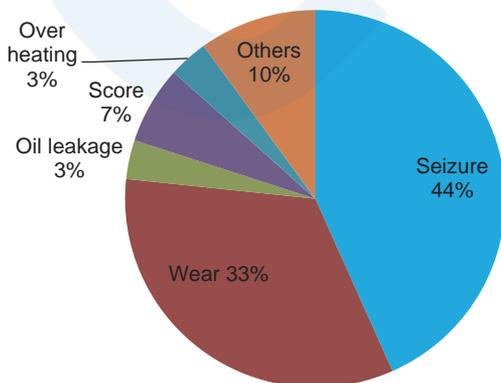
Fig. 11 Breakdown of type of damage for fuel injection pump
