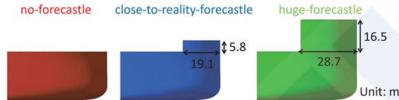
図8 Side view with assumed forecastle shape model based on BC-10
