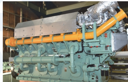
Fig. 10 Medium-speed, four-stroke 28ADF engine for A-Tug (power: 1618 kW/750 rpm/unit, D/S: 280/390 mm, 6 cylinders, Pme: 1.8 MPa) 18)
