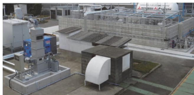
Fig. 7 J-ENG's single-cylinder ammonia test engine (left) and ammonia supply system (right) 15)
