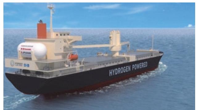
Fig. 13 Hydrogen-fueled multi-purpose vessel (17,500 DWT type) (Rendering) 24)
