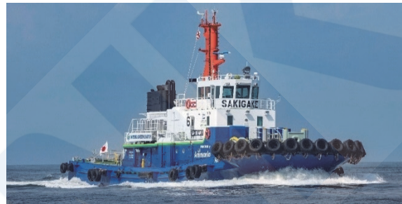
Fig. 9 A-Tug "Sakigake" (main engine output: 1618 kW x 2 units) 19)
