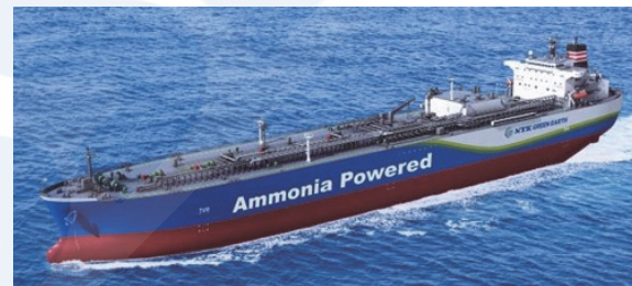
Fig. 6 AFMGC: Ammonia-fueled medium gas carrier (projected figure) 14)
