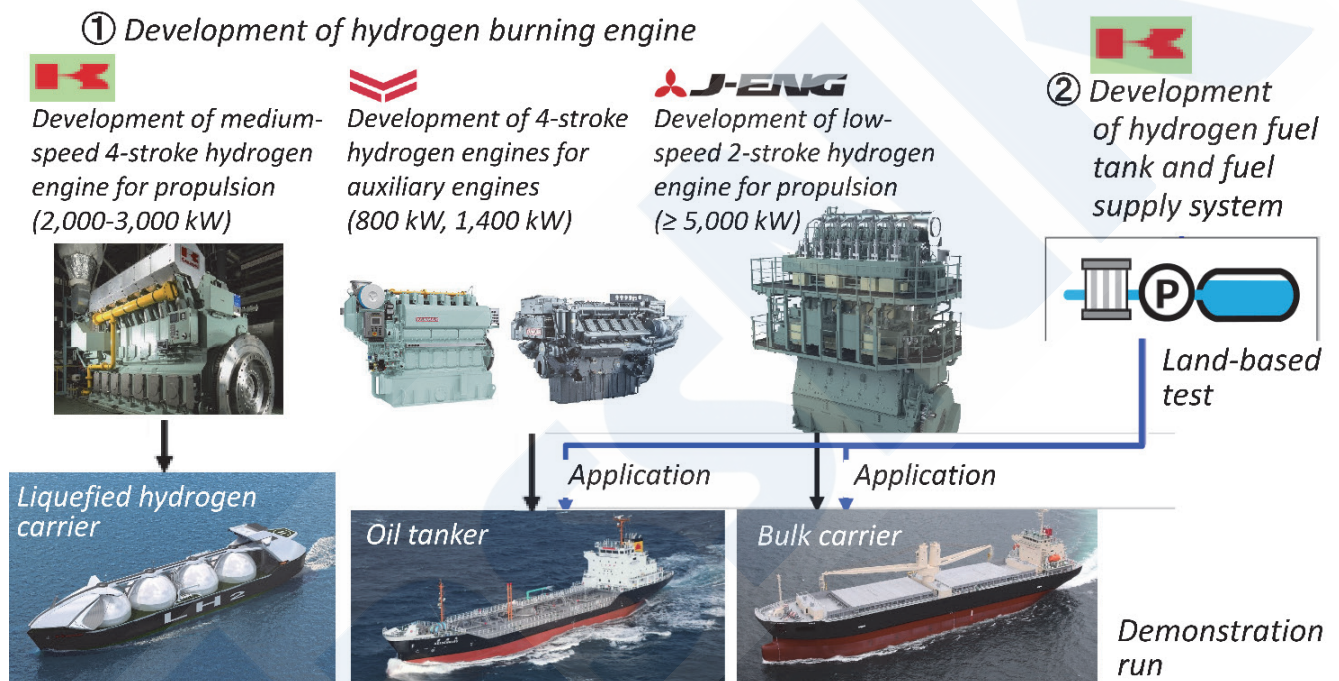
Fig. 11 Development of marine hydrogen engine and MHFS (Marine Hydrogen Fuel System) (NEDO website)
