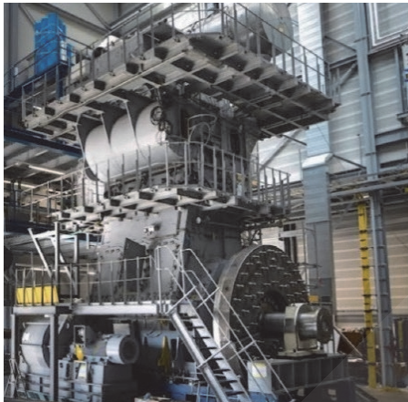
Fig. 8 WinGD's low-speed, two-stroke, single cylinder test engine (cylinder diameter: 520 mm) (courtesy of WinGD)
