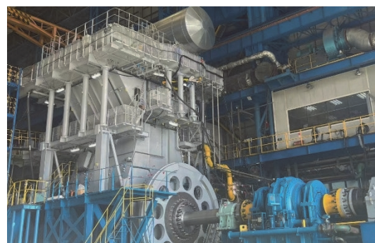
Fig. 2 Single-cylinder test engine SCE920 (cylinder diameter: 920 mm) for WinGD's low-speed, two-stroke methanol engine development (courtesy of WinGD)
