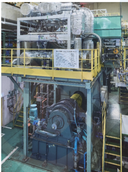
Fig. 7 J-ENG's single-cylinder ammonia test engine (left) and ammonia supply system (right) 15)
