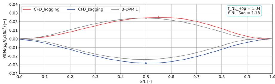
(b) CFD+MLRW, Vertical bending moment distribution along the ship length
