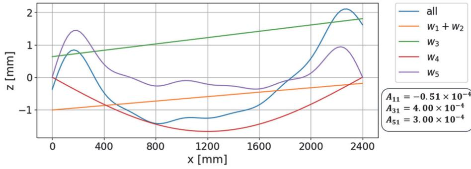
Fig. 8 Initial deflection with two peaks near both ends
