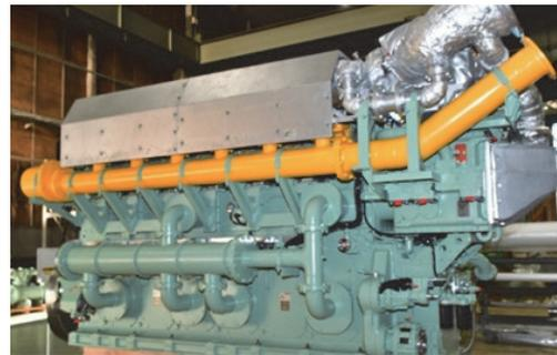
Fig. 10 Medium-speed, four-stroke 28ADF engine for A-Tug (power: 1618 kW/750 rpm/unit, D/S: 280/390 mm, 6 cylinders, Pme: 1.8 MPa)<sup>18)</sup>
