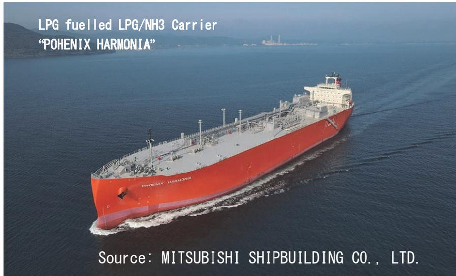
Fig. 4 LPG-fueled LPG/ammonia carrier, M/V PHOENIX HARMONIA
