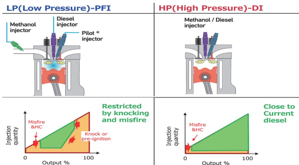
Fig. 3 Two combustion patterns for medium-speed, four-stroke methanol engines<sup>7)</sup>
