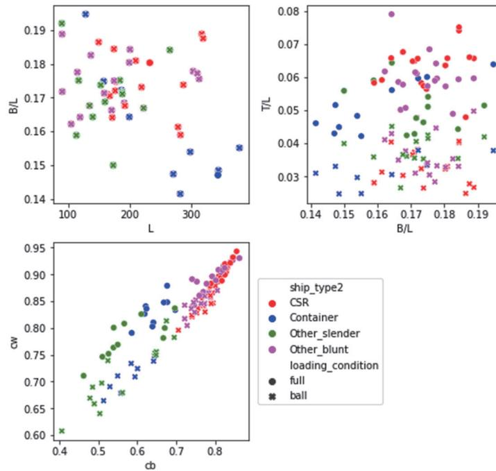
Fig. 1 Principle particular of target ships (circles: Full load condition, crosses: Ballast condition)
