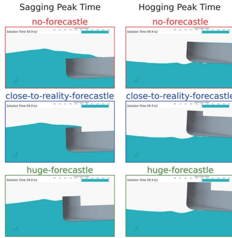
Fig. 10 Comparison of green water on deck at the time of maximum hogging and minimum sagging moment (Bulk carrier, BC-10, Full load condition)
