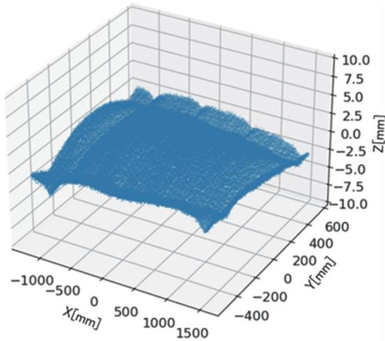
Fig. 2 Point cloud data after coordinate transformation
