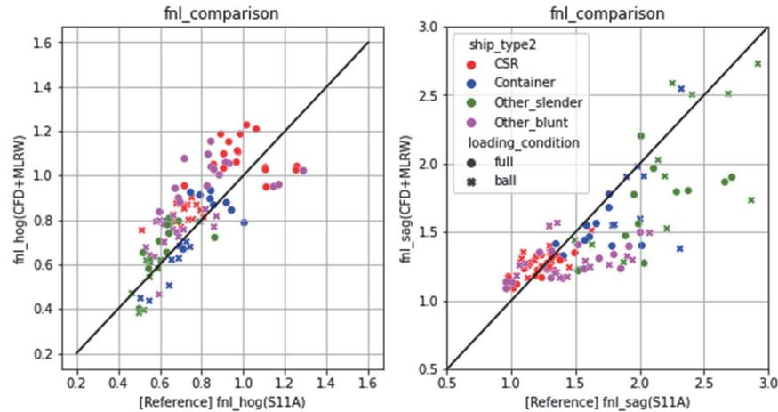
Fig. 15 Comparison with non-linear factor specified in IACS UR S11A (as reference), (left): hogging, (right): sagging.
