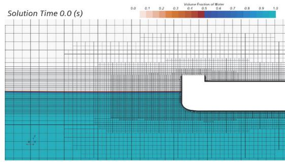
Fig. 5 VOF distribution of BC-10 with mesh diagram at initial condition (side view, near the bow)
