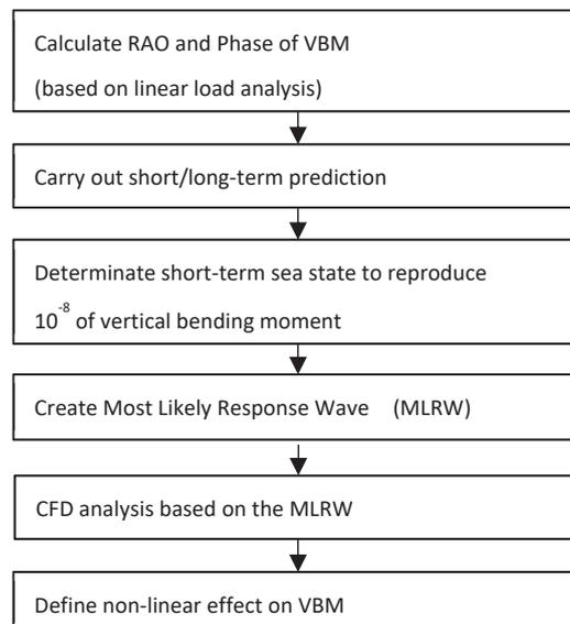
Fig. 2 Flowchart to reproduce vertical wave bending moment in extreme seas and define non-linear effect on the moment
