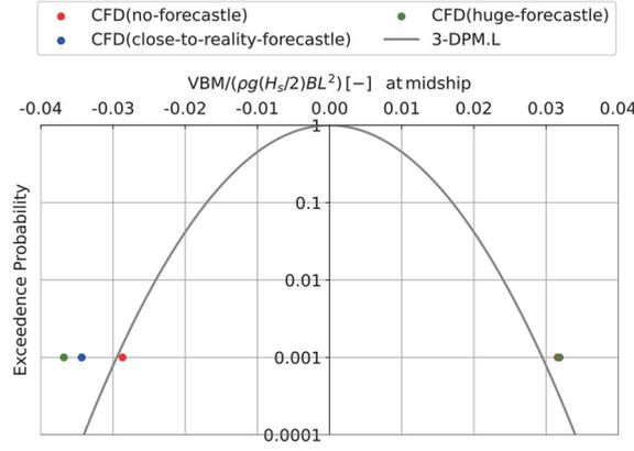
Fig. 9 The effect of with/without forecastle on vertical wave bending moment at midship (Bulk carrier, BC-10, Full load condition)
