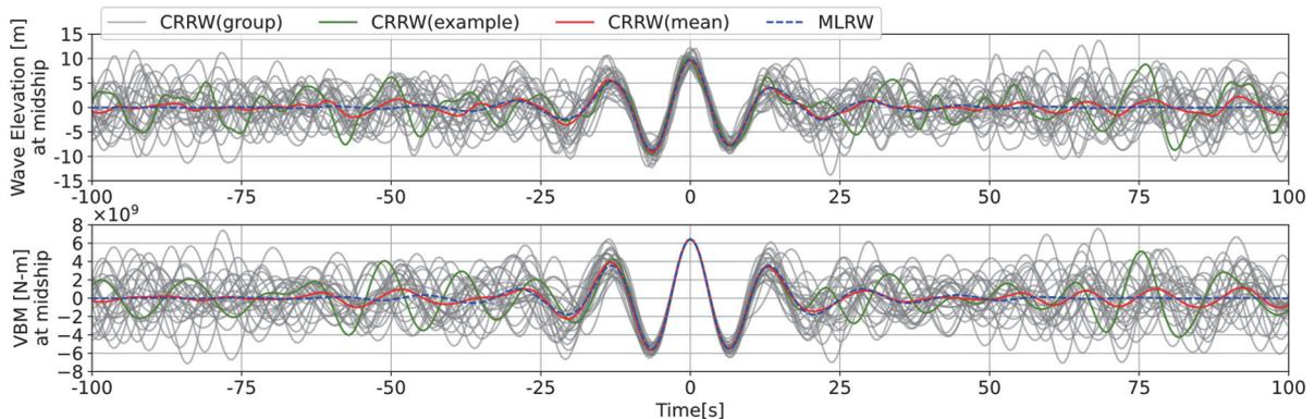
Fig. 3 An example of wave elevation and vertical bending moment in CRRW and MLRW (Bulk carrier, BC-10, Full load condition)
