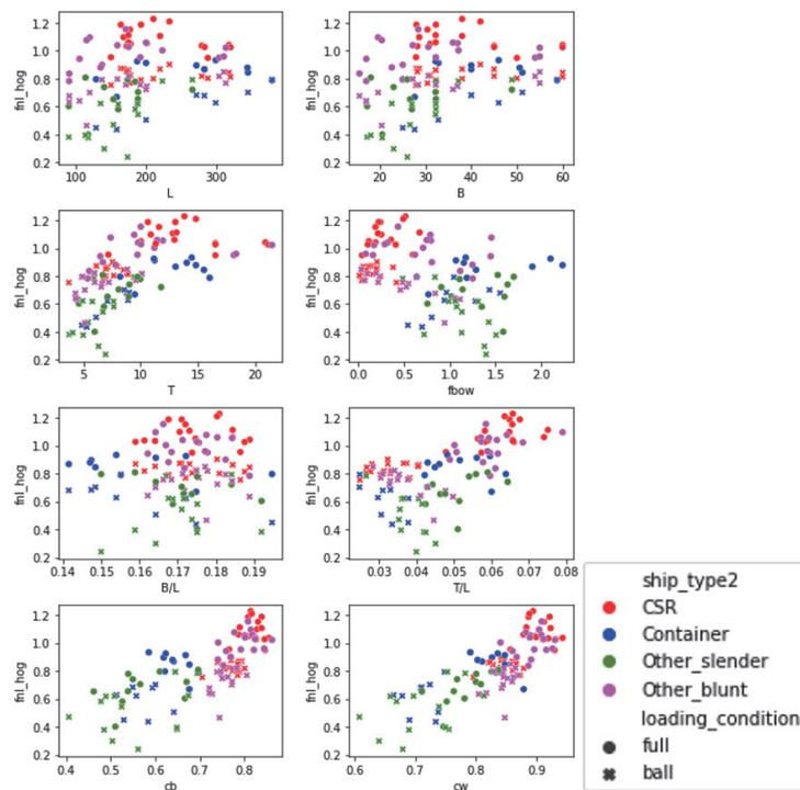
Fig. 11 Sensitivity of non-linear effect coefficient to principal particulars of ships, hogging moment
