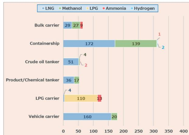
Fig. 7 Trends in alternative fuel ships on order (by ship type)
