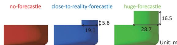
Fig. 8 Side view with assumed forecastle shape model based on BC-10
