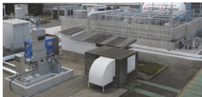
Fig. 7 J-ENG's single-cylinder ammonia test engine (left) and ammonia supply system (right)<sup>15)</sup>
