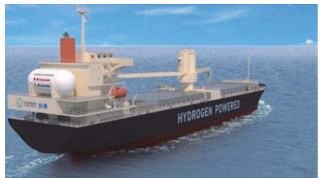
Fig. 13 Hydrogen-fueled multi-purpose vessel (17,500 DWT type) (Rendering)<sup>24)</sup>
