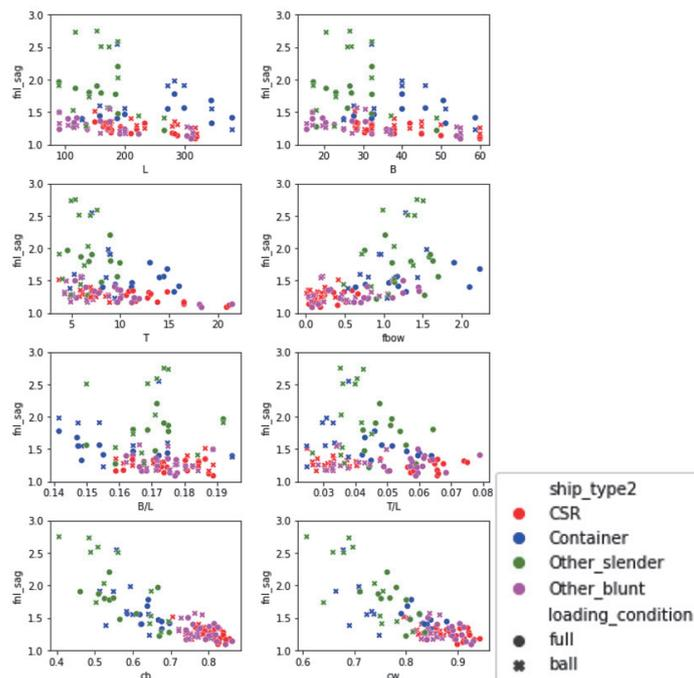
Fig. 12 Sensitivity of non-linear effect coefficient to principal particulars of ships, sagging moment
