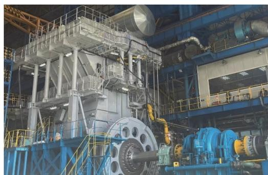
Fig. 2 Single-cylinder test engine SCE920 (cylinder diameter: 920 mm) for WinGD's low-speed, two-stroke methanol engine development (courtesy of WinGD)
