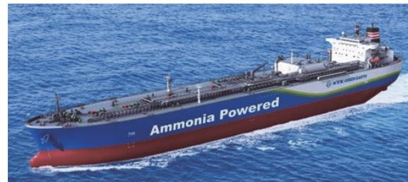
Fig. 6 AFMGC: Ammonia-fueled medium gas carrier (projected figure)<sup>14)</sup>
