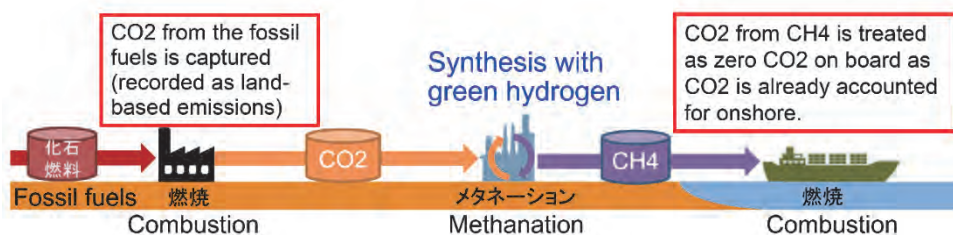
Fig. 2 Example of carbon-neutral methane production route 1)
