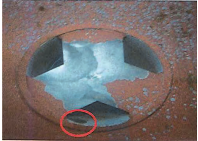
Fig. 3 Corrosion around welded parts between distance piece and bluff body
