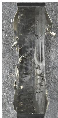
Fig. 8 Bearing metal surface after simulation test
