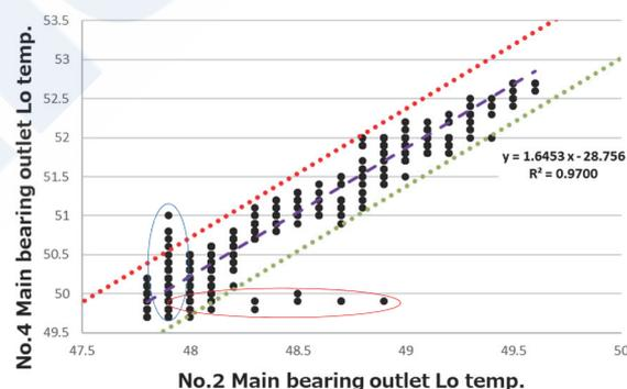
Fig. 3 Correlation plot chart for LO outlet temperatures of main bearings No. 2 and No. 4 (December)
