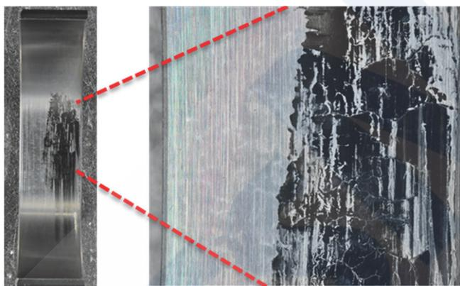
Fig. 10 Bearing metal surface after seizure confirmation test
