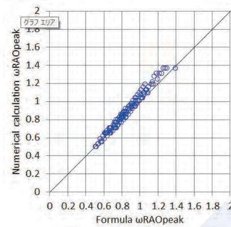
Figure 10 Comparison of  $\omega_{RAOp_{eak}}$  of heave acceleration between equation (21) and numerical calculation
