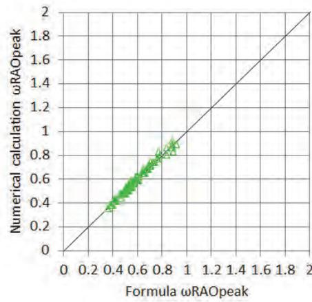
Figure 12 Comparison of  $\omega_{RAOPeak}$  of pitch angle between equation (21) and numerical calculation
