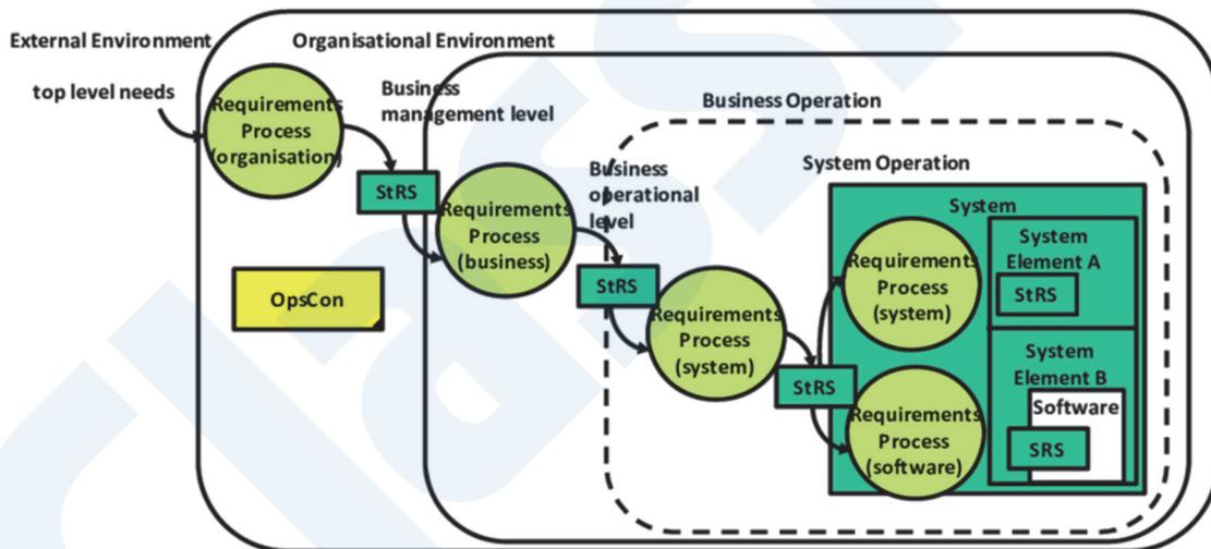
Figure 2 Example of requirement definition process flow and corresponding requirement specifications (Source: ISO / IEC / IEEE 29148)
