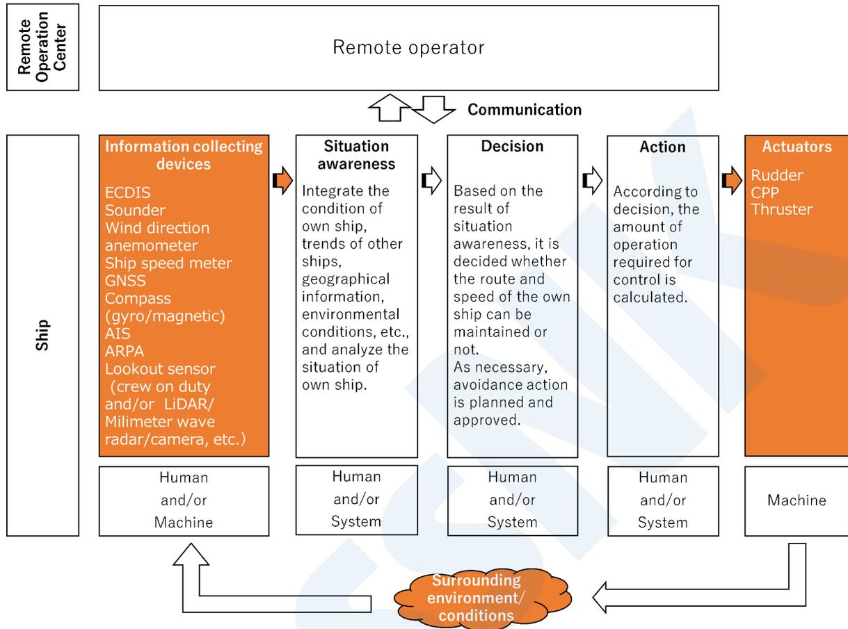
Figure 5 Image of maneuvering operation on an autonomous ship
