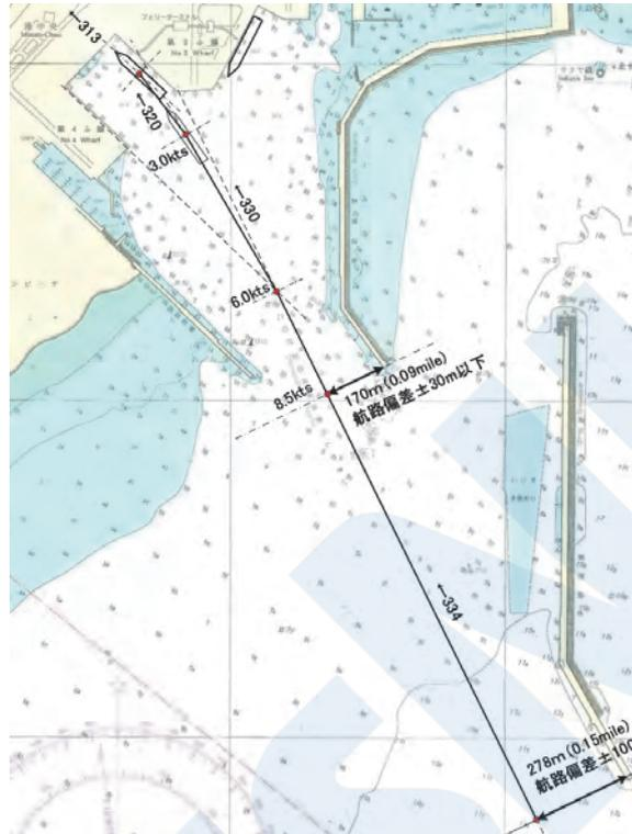
Figure 10 Maneuvering scenario used in demonstration test
