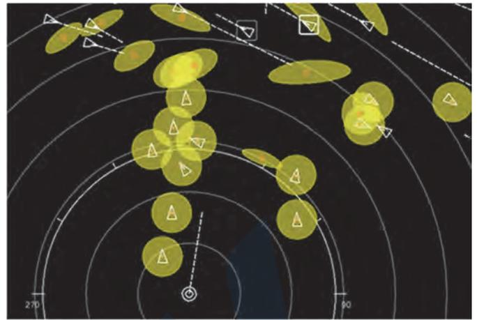
Figure 34 Example of DAC display (transparent fill)
