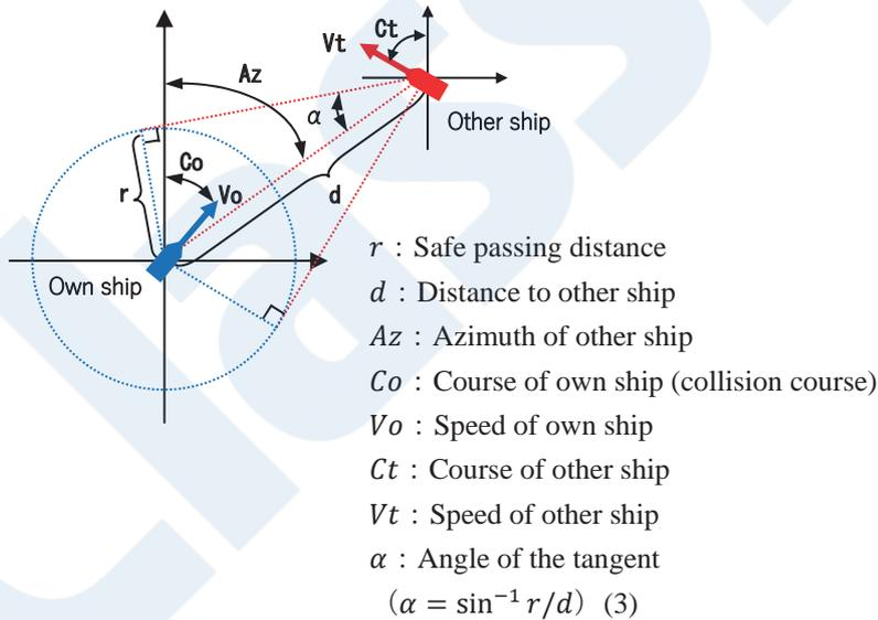
Figure 16 Collision course calculation diagram
