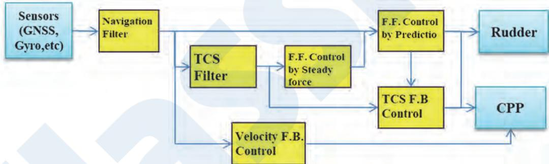
Figure 4 Block diagram of approach maneuvering control functions
