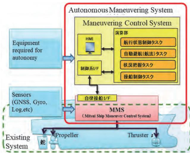
Figure 2 Configuration of autonomous maneuvering system
