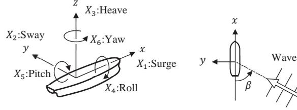
Figure 1 Definitions of coordinate system, motion and incident wave
