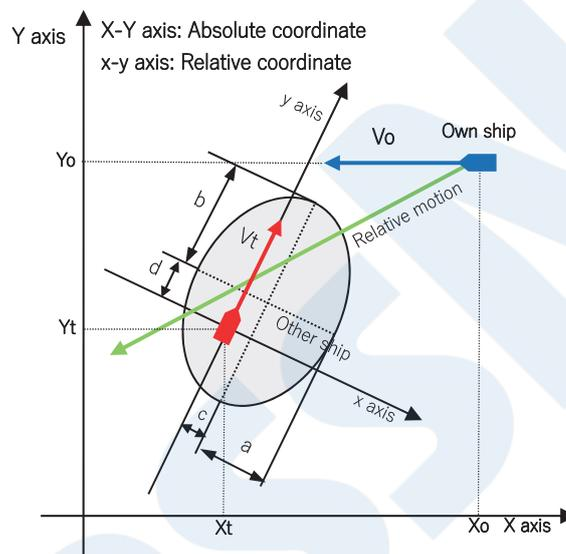
Figure 13 Concept of safe passing distance
