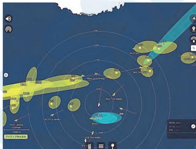
Figure 35 Example of DAC display on “Aisea PRO”
