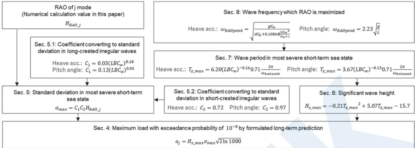
Figure 1 Flow diagram for formulated long-term prediction
