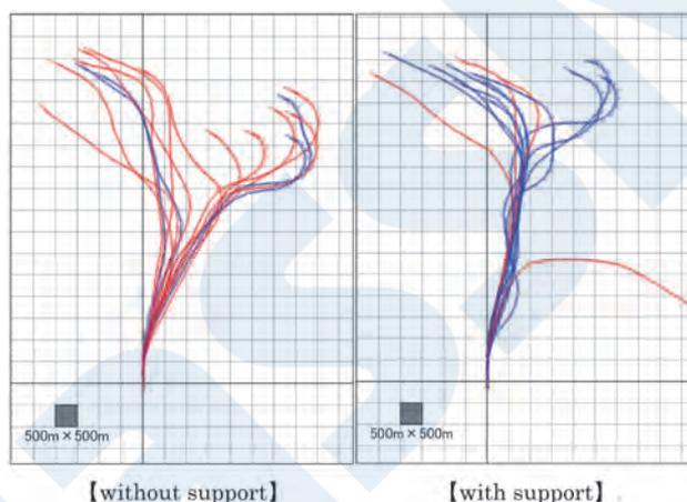
Figure 38 Track charts showing ship handling results
