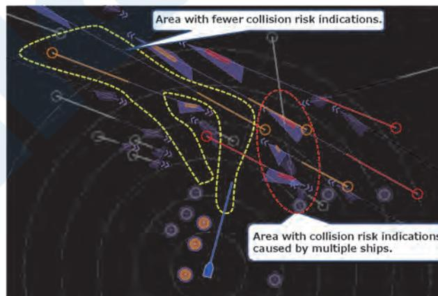
Figure 12 Collision risk indications established for this system
