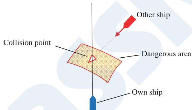
Figure 20 Example of calculation of dangerous area
