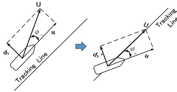
Figure 7 Image of control for steady external force
