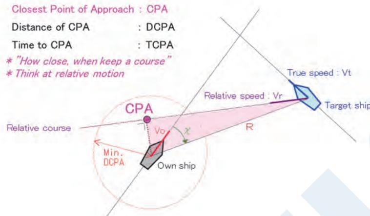
Figure 1 Information based on close point of approach
