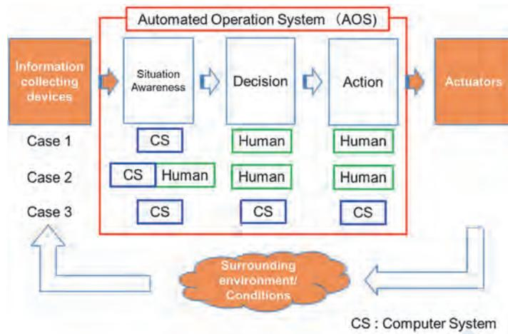
Figure 1 Conceptual diagram of Automated Operation System
