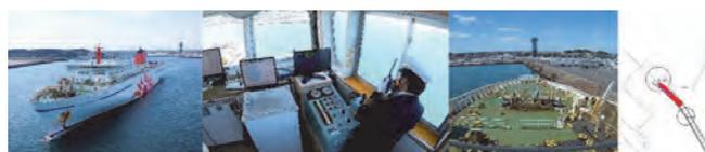
Figure 8 Scenes from automatic pier docking and undocking simulation and demonstration experiment with large-scale car ferry, *Sun Flower Shiretoko*<sup>16)</sup>
