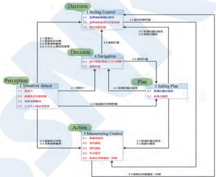
Figure 3 Task block diagram of autonomous maneuvering control functions
