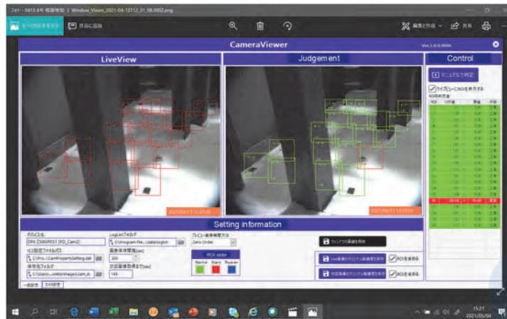
Figure 7 FO Leak Detection System
