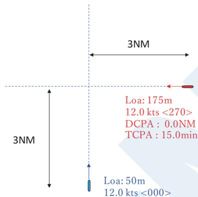
Figure 4 Example of test scenario (1:1 crossing ship)
