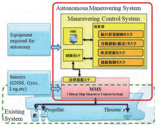
Figure 2 Configuration of autonomous maneuvering system
