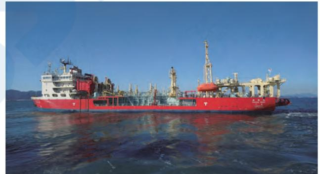
Figure 6 Combined dredger-and-oil recovery ship, *Kaisho Maru*
