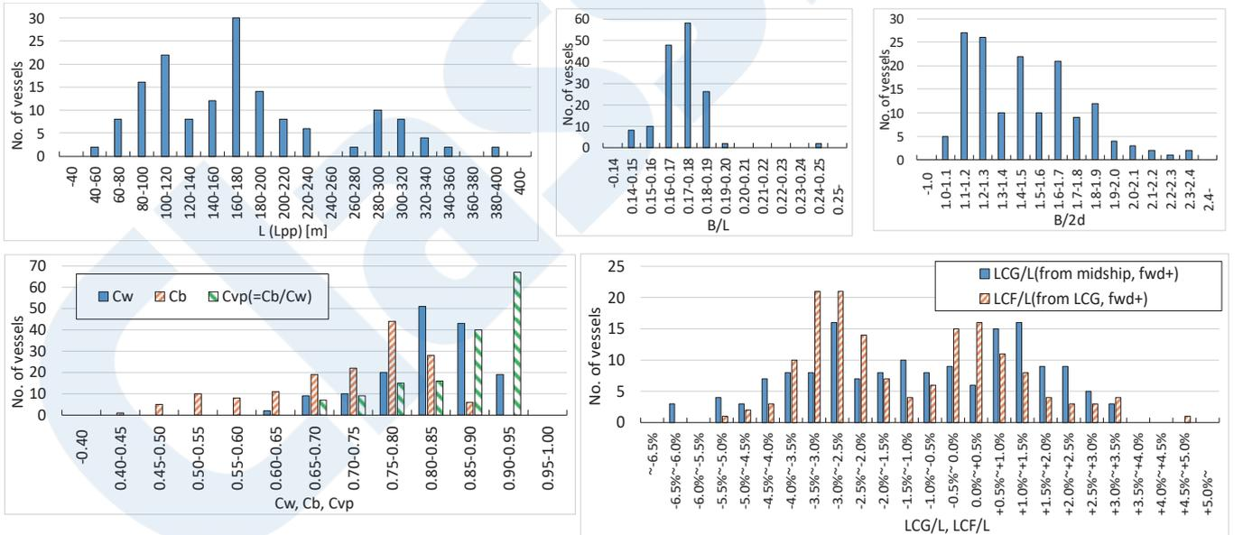
Figure 2 Histogram of hull-form parameters of target ships.
