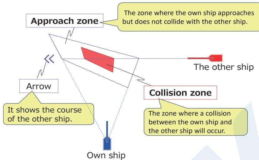
Figure 11 Display of collision risk indications (approach zone and collision zone)
