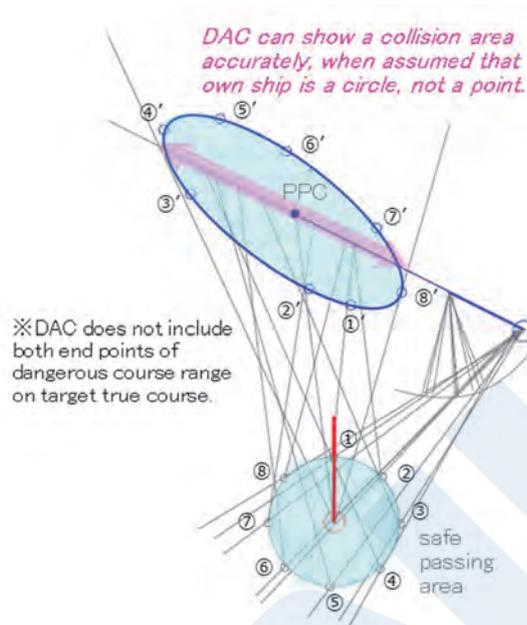
Figure 29 Principle of DAC (case of octagonal DAC)
