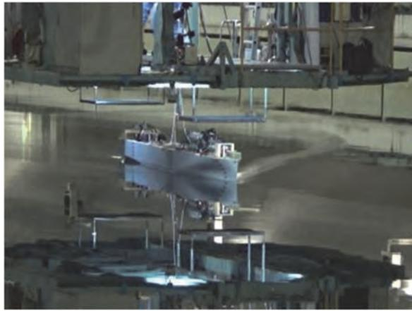
Figure 5 Autonomous Berthing Maneuvering System – Model Test
