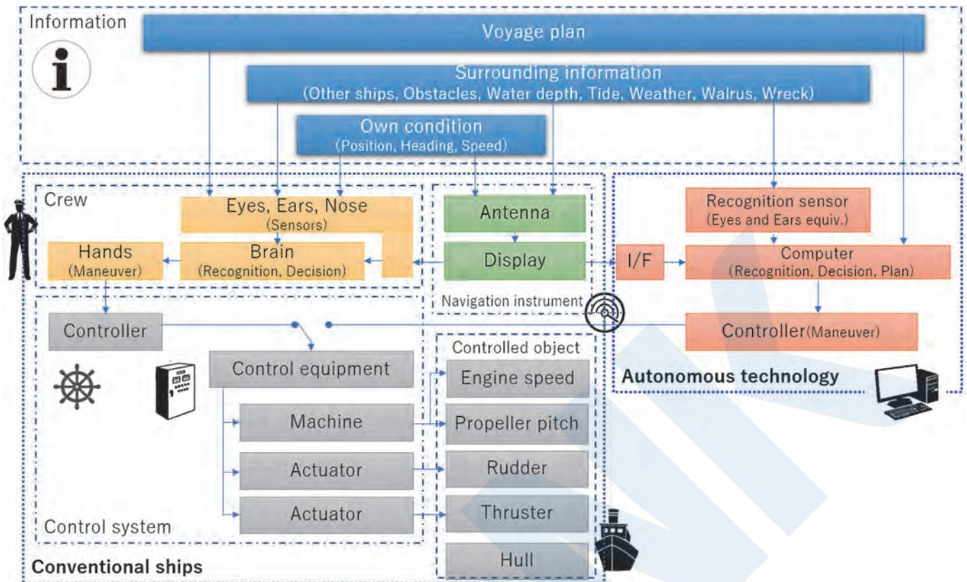
Figure 3 Differences with existing ships in service
