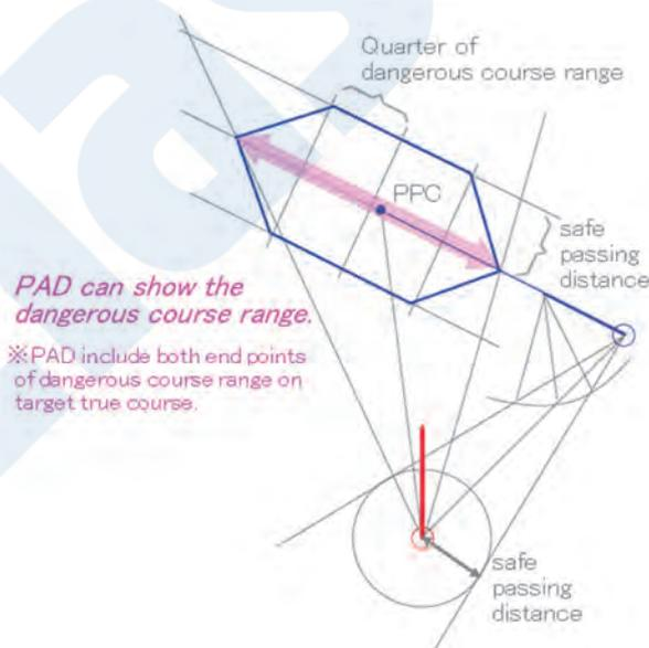
Figure 28 Principle of PAD (case of hexagonal PAD)
