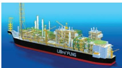
The LiBro® FLNG concept is based on existing shipbuilding standards allowing it to be fitted topside of standard hull sizes. Fitted on a 300m x 50m vessel, the technology can produce up to 2 million tons of LNG annually, and store up to 160,000m<sup>3</sup> of LNG and 20,000m<sup>3</sup> of condensate. To enhance its early delivery and cost-effective features, LiBro® FLNG can be applied to both new built hull and existing hull conversions.
