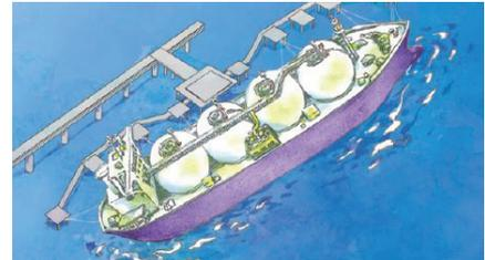
LNG receiving terminals. Regasification facilities fitted on LNG carriers can replace the role of onshore LNG storage tanks and regasification facilities, which require huge onshore construction work, as well as environmental assessments.
