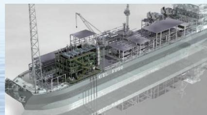
which has been developed by a joint R&D venture between MODEC and TOYO. The GTL itself converts associated gases from oil fields into syncrude. Until now, producers would flare these associated gases or reinject into subsea reservoirs for safety reasons. However, the process is either harmful to the
