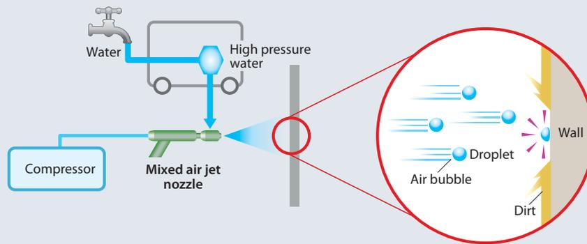
Fig. 1 Principle concept of *Konki-jet* system.
