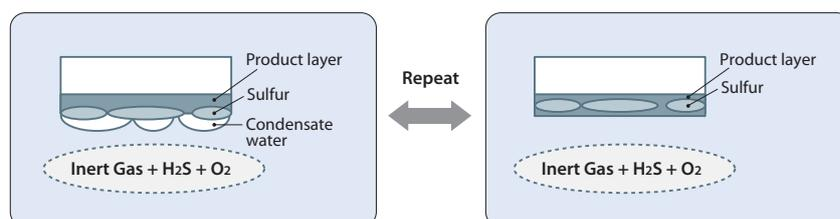
Fig.2 Corrosion mechanism at upper deck plate.
