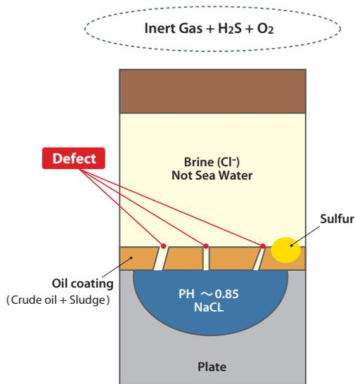
Fig.3 Corrosion mechanism at inner bottom plate.
