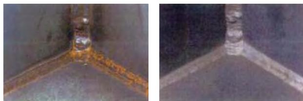
(a) Weld bead (internal corner) before treatment (b) Weld bead (internal corner) after treatment
