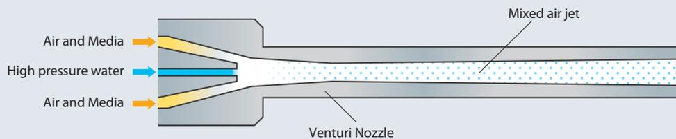
Fig. 2 Schematic cross-section of *Konki-jet* nozzle.
