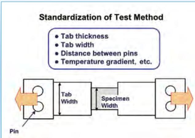
Basic concept of brittle crack arrest toughness Kca test.
