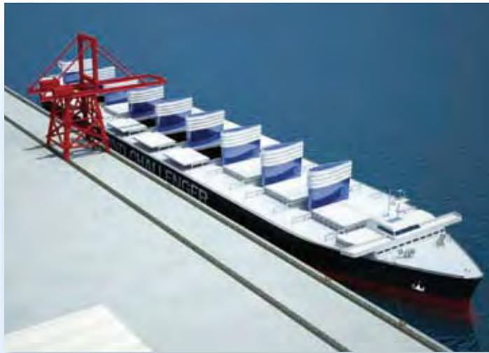
Fig. 2: Wind driven bulk carrier in port. (Courtesy University of Tokyo.)
