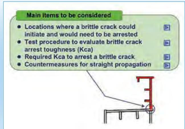
Key points to consider in the development of an effective brittle crack arrest design.
