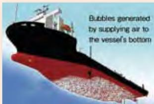
Image from the bottom of a module carrier equipped with an air lubrication system. (Source: MHI News Release, 24 Feb. 2010.)
