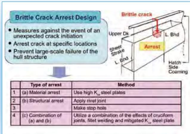
Basic concept of brittle crack arrest design.
