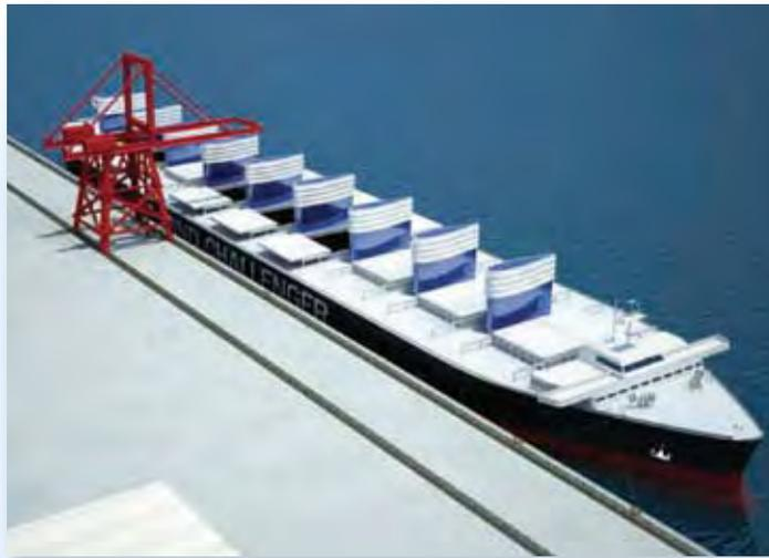
Fig. 2: Wind driven bulk carrier in port. (Courtesy University of Tokyo.)
