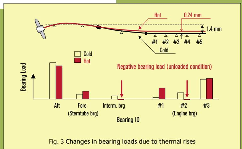
The most important point in NK's new alignment guidance is to introduce the following calculation conditions, which cause changes in bearing offsets:
