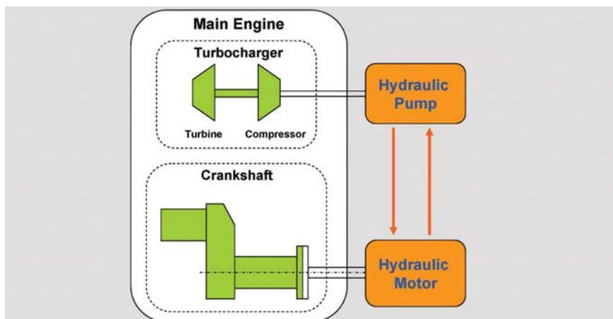
Concept of the THS; Hydraulic pump: Take out excess energy of exhaust gas from the Turbocharger Hydraulic motor: Assists rotation of crank shaft with recovered hydraulic power
