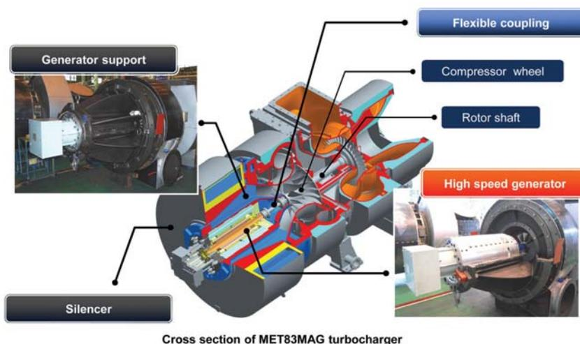
Cross section of MET83MAG turbocharger
