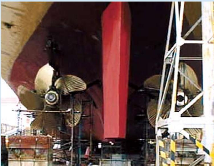
Photo4:Conversion of a high speed car ferry to a NHV propeller
