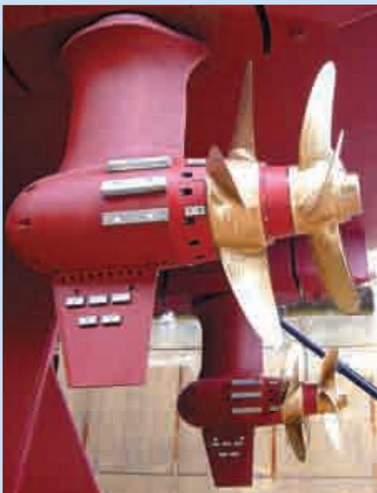
Photo1:Podded contra-rotating propeller propulsion system
