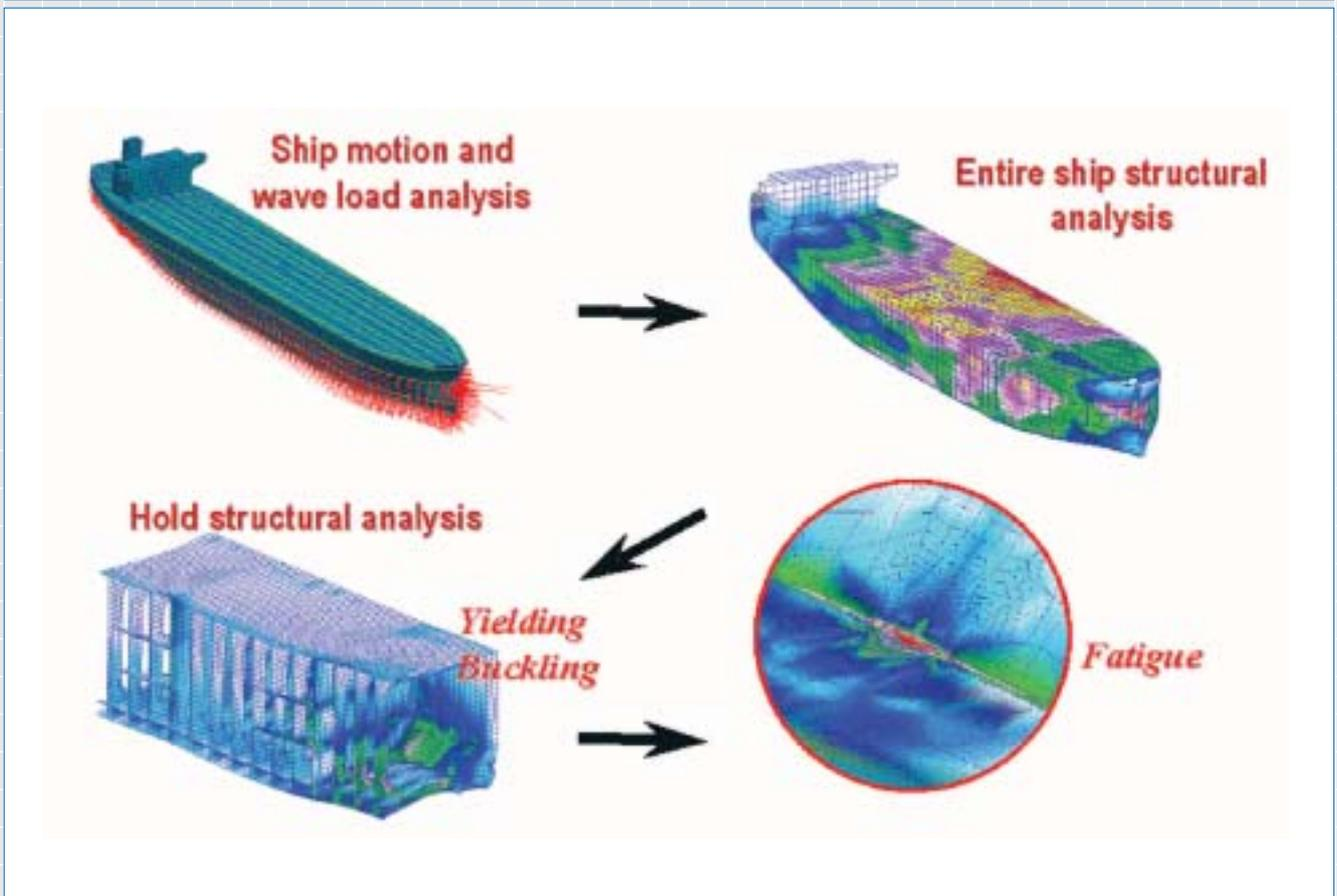
Structural Analysis and Validation System, ASSAS, supports PrimeShip Total Strength Assessment. This is the most rational design and assessment of hull structures, based on the total analysis concept for each ship, and based on direct calculation of wave-induced dynamic loads, global and local structural analysis and strength assessment against yielding, buckling and fatigue (Yoneya et al., 2001).
