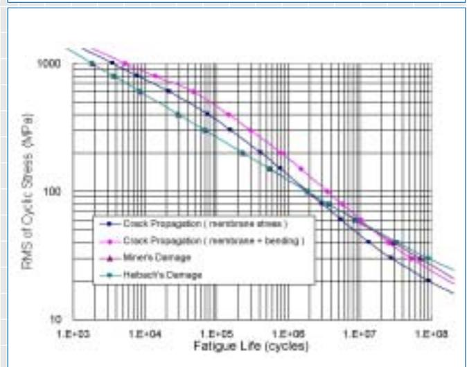
design S-N curves have been adopted for welded parts and non-welded parts, based on the UK-DOE curves (Figure 6). The effect of structural mean stress on fatigue strength is taken into account in a practical and rational manner, based on calibration with fatigue damage experience in side longitudinals of oil tankers (Yamamoto & Matsuoka, 2001). Design loads and structural analysis methods generally conform to the *Guidelines for Direct Strength Analysis*.
