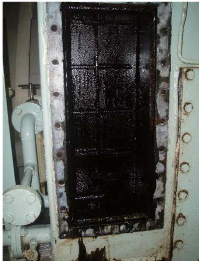
Oily inside of oil water separator
