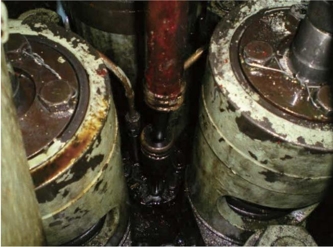
Partial lack of a high-pressure fuel oil pipe doubling jacket
