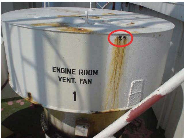
Corrosion holes in the casing of ventilator
