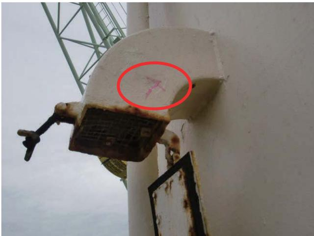
Hole with inappropriate repair with tapes
