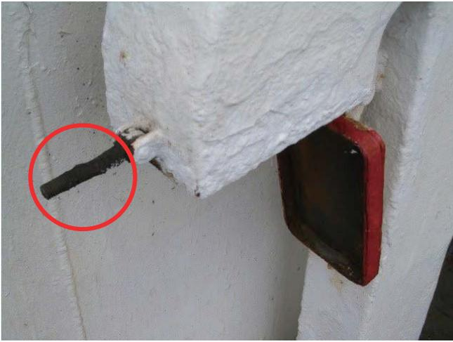
Missing butterfly nut of gooseneck ventilator
