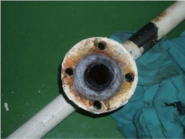
Oily inside of discharge pipe
