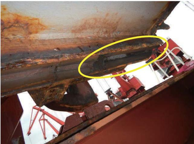
Partly missing rubber packing
