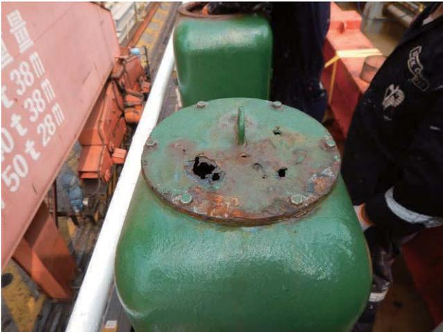
Corrosion holes in air pipe head
