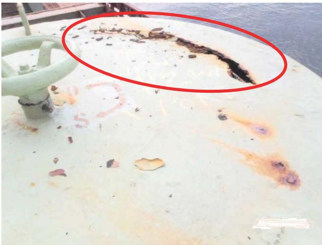
Corrosion holes in the casing of ventilator
