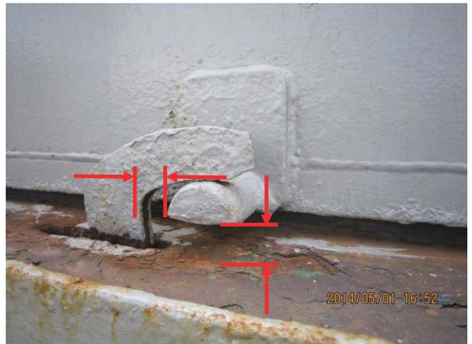
Excessive gaps of hatch cover
