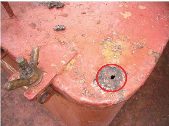
Corrosion hole in access hatch
