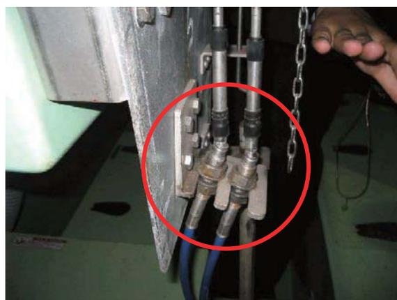
Bent release cable and bracket
