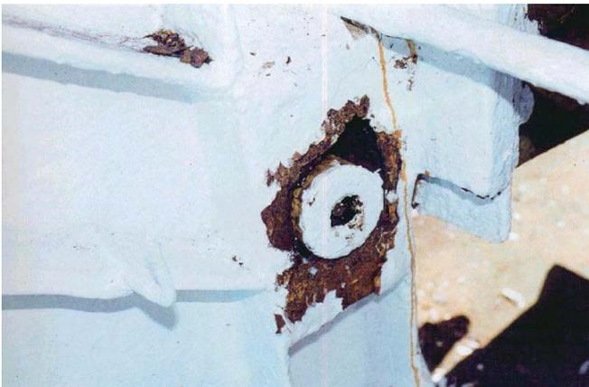
Housing wasted around carrying hinge pin
