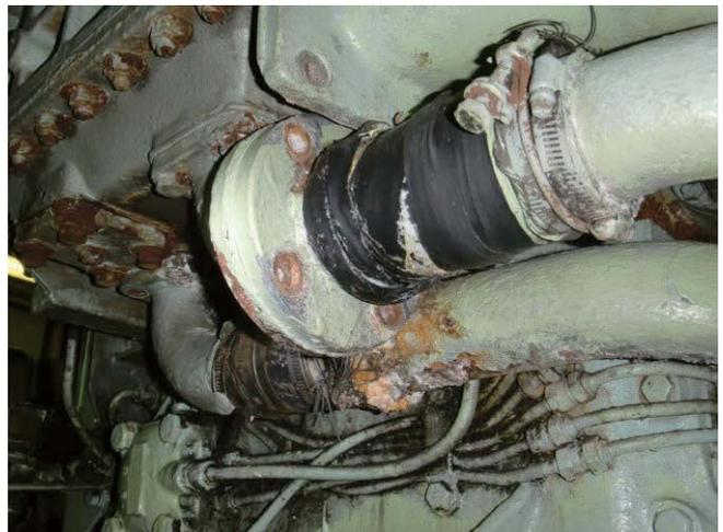
Inappropriate repairs by rubber patch on SW pipe for G/E
