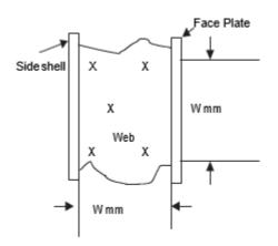
Figure 3 Typical 5 point pattern on the web plate
