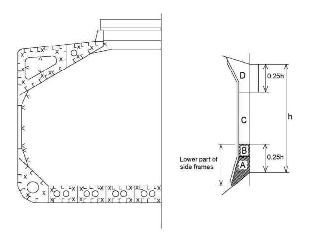
Note: The gauging pattern for web plating is to be a three point pattern for zones A, C and D, and a two point pattern for zone B (see figure). The gauging report is to reflect the average reading. The average reading is to be compared with the allowable thickness. If the web plating has general corrosion then this pattern is to be expanded to a five-point pattern.
