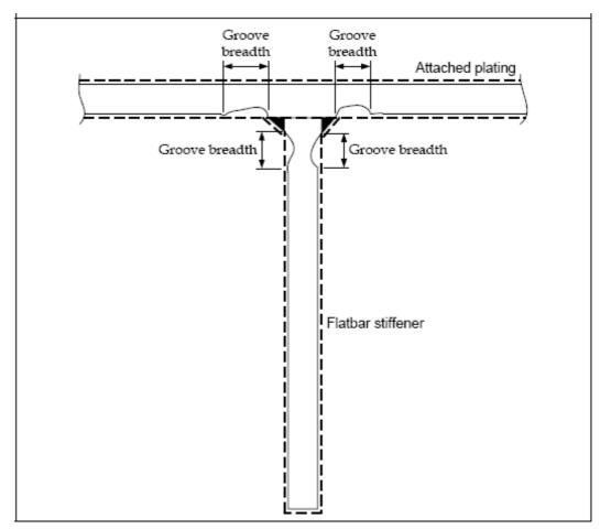
Figure 3 - Grooving corrosion
