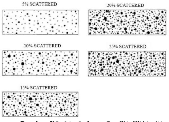
Figure 2 Pitting intensity diagrams (from 5% to 25% intensity)
