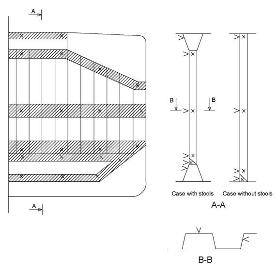
Note: Measurements to be taken in each shaded area as per views A - A and B - B
