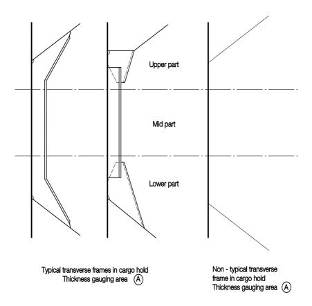
4. The remaining corrosion addition is to be recorded with result of gauged thickness minus renewal thickness. If the result is negative, the structure in way shall be renewed, and the mark "R" is to be indicated in the right-hand column. If the result is between 0 and 0.5 mm (0 included), the structure in way shall be additional gauged, and the mark "S" is to be indicated in the right-hand column.
