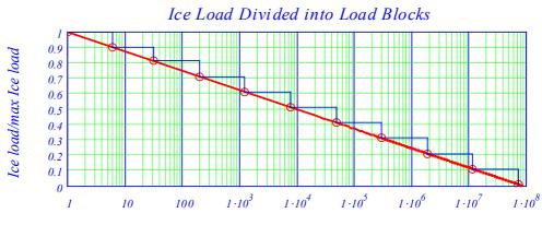
Figure 8: Example of ice load distribution (spectrum) for the shafting (k = 1)
