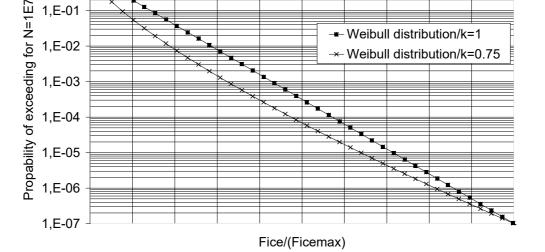
Figure 2: The Weibull-type distribution (probability that  $F_{ice}$  exceeds  $(F_{ice})_{max}$ ) that is used for fatigue design.
