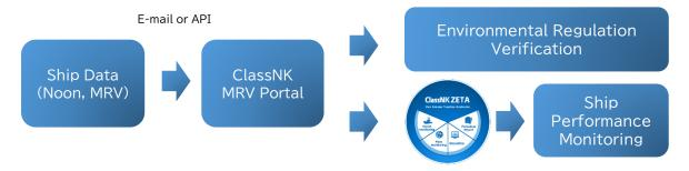
3. You can get the most recent ship performance analysis automatically. Every time new ship data is received, the model is automatically update.
