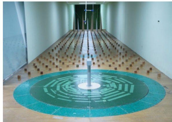
b) Installation of turbulent boundary layer generator
