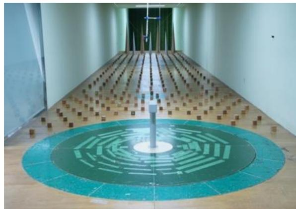
b) Installation of turbulent boundary layer generator
