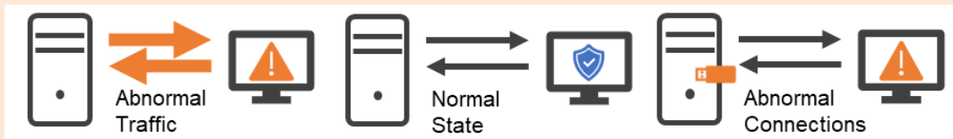
Figure 1.4 Alarms triggered by unintended network activities
