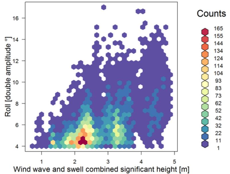
Figure 7. Bivariate histogram for roll amplitude vs. wave height.
