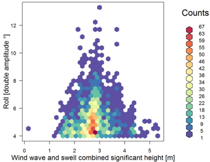
Figure 6. Bivariate histogram for roll amplitude vs. wave height
