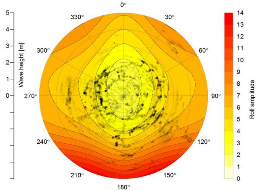
Figure 9. Polar diagram for roll amplitude
