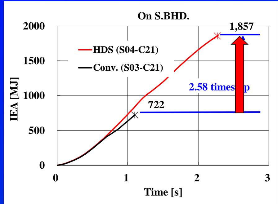
Energy absorption by the struck ship until oil tank rupture becomes about 2.6-2.9 times larger than conv.
