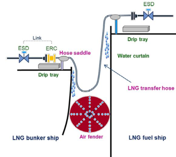
**Arrangement of LNG bunkering equipment (example of STS)**
