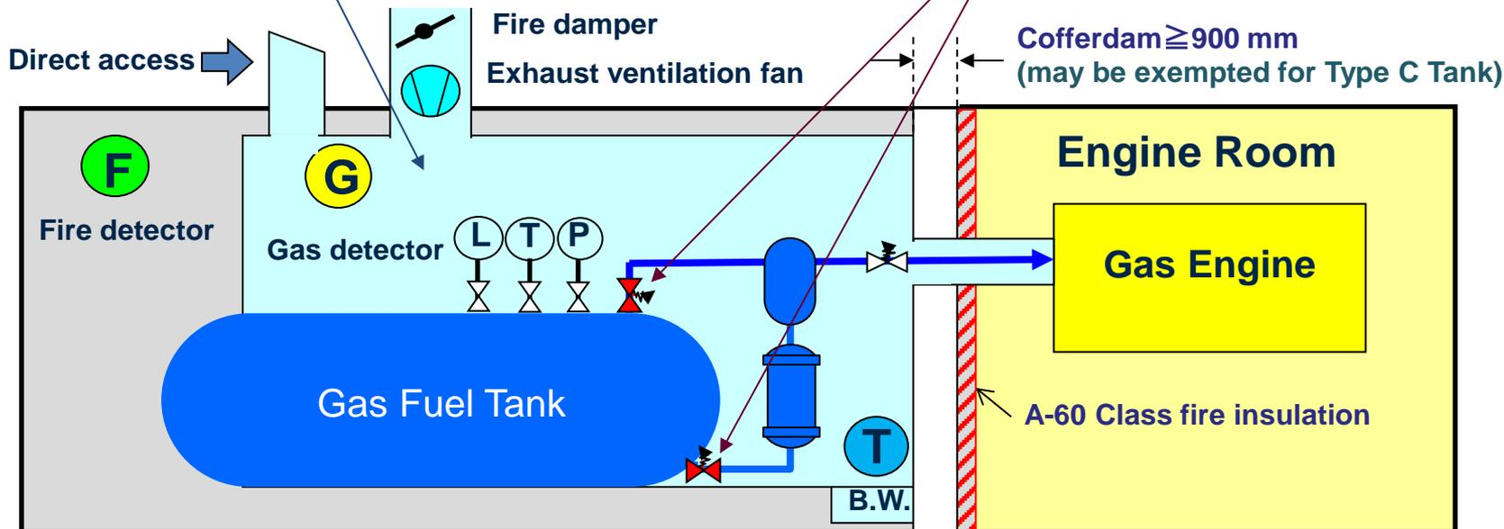
**Major requirements : *Fuel Supply to & inside Engine Room 1/3*****Gas Safe Machinery Space**
