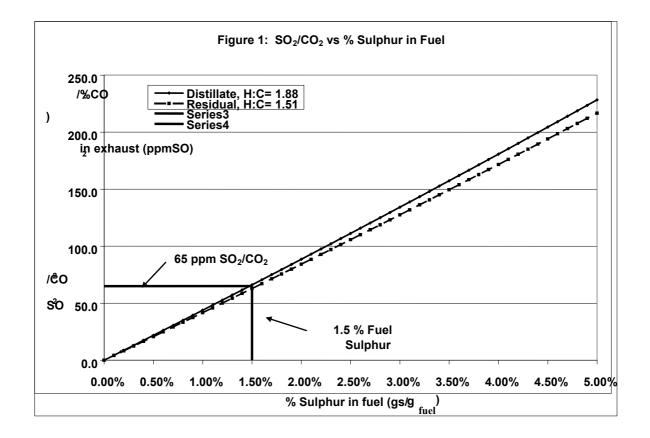
2 Correspondence between 65  $(^{1}ppm/\%)$  / CO<sub>2</sub> and 6.0 g/kWh is demonstrated by showing that their S/C ratios are similar. This requires the additional assumption of a brake-specific fuel consumption value of 200 g/kWh. This is an appropriate average for marine diesel engines. The calculation is as follows:
