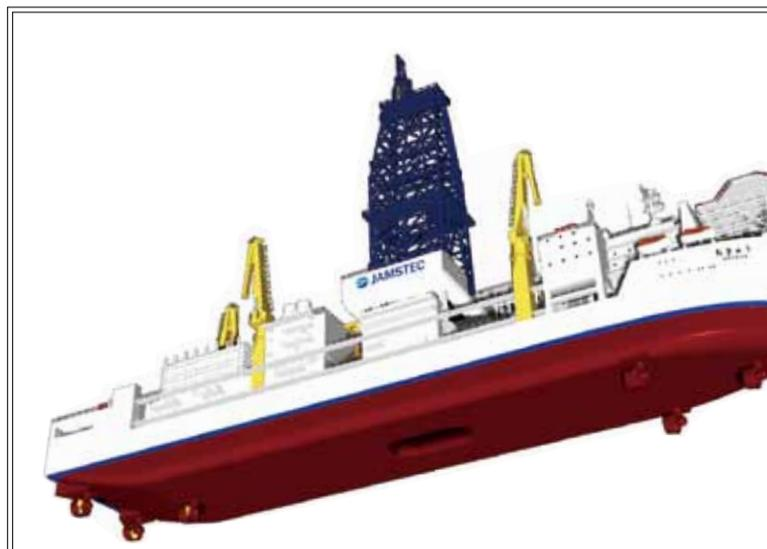
CHIKYU uses GPS position data from satellites and acoustic position data from transponders on the sea floor to confirm its position.
