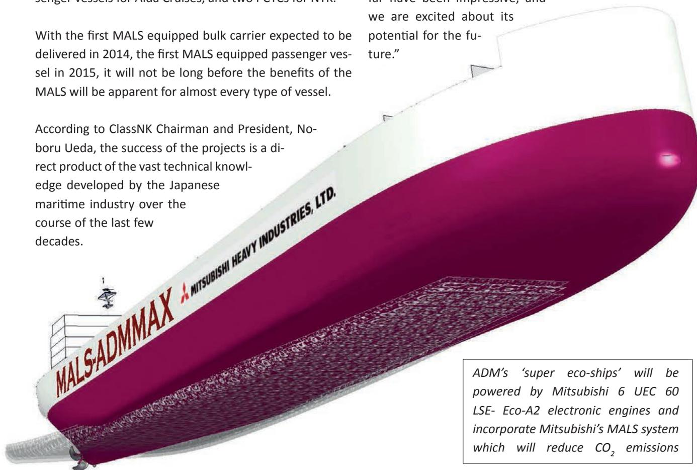
ADM's 'super eco-ships' will be powered by Mitsubishi 6 UEC 60 LSE- Eco-A2 electronic engines and incorporate Mitsubishi's MALS system which will reduce CO<sub>2</sub> emissions
