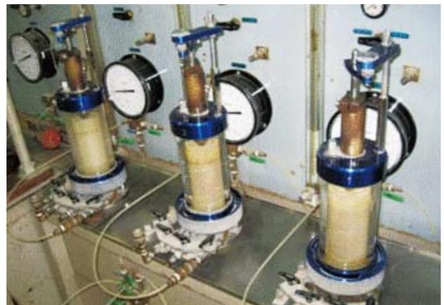
Tri-axial compression Test
