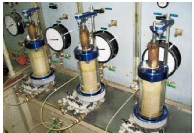
Tri-axial compression Test
