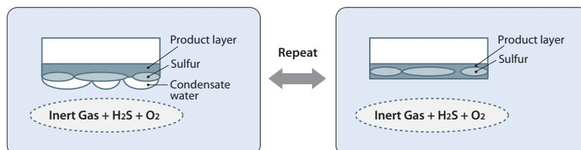
Fig.2 Corrosion mechanism at upper deck plate.
