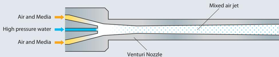
Fig. 2 Schematic cross-section of *Konki-jet* nozzle.
