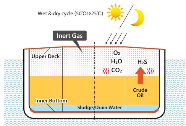
Fig. 1 Overview of corrosion mechanism in cargo oil tank.
