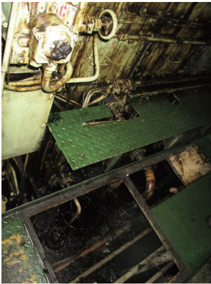
Oil leakage and accumulation
