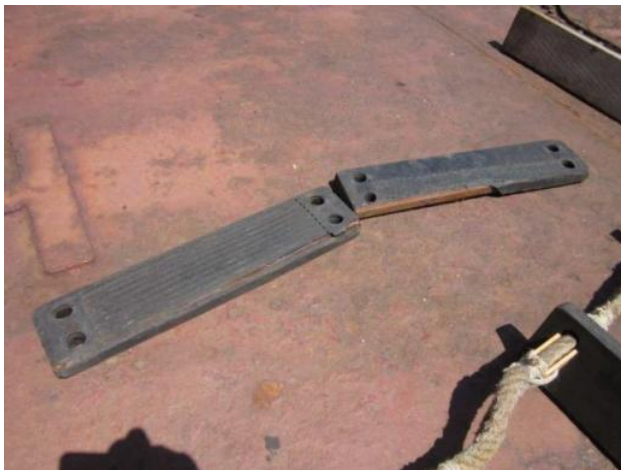
Broken pilot ladder.
