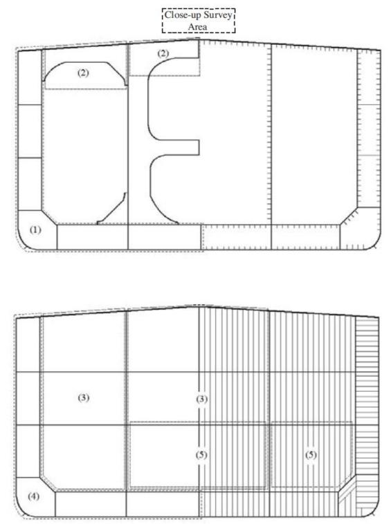
Figure 9 - Close-up Survey Requirements for Double Hull Oil Tankers Areas (1) to (5)
