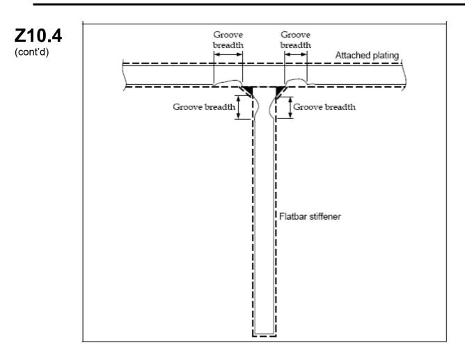
Figure 3 - Grooving corrosion
