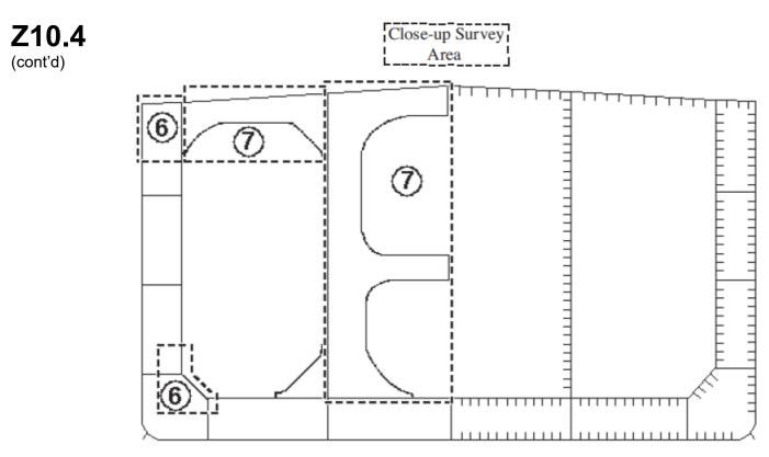
Figure 10 - Close-up Survey Requirements for Double Hull Oil Tankers Areas (6) and (7)
