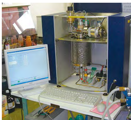
Combustion test using FIA-100FCA (Standard: IP541/06)
