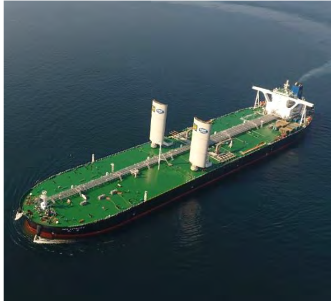
A VLCC with a pair of “hard airfoil sails” developed by Dalian Shipbuilding Industry of CSIC with New Vitality (2018)
