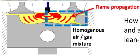
How is the flame propagation and abnormal combustion in <u>lean-burn type gas engine</u>?
