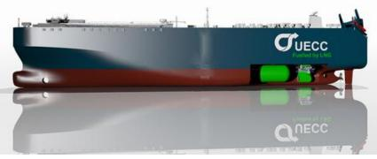
• United European Car Carriers (UECC) jointly owned by NYK and Wallenius Lines has ordered KHI two PCCs propelled by MAN low-speed ME-GI gas (DF) engine. (for voyage in European ECA)
