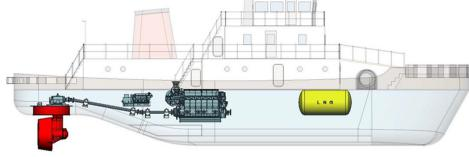
LNG Fuel Tank25m3 (12.5m3 X 2), bunkering : once a weekPropulsion SystemDF Engine (abt.2000kW ) & direct coupling with thruster X 2sets
