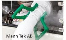
Note: In case where BAC is used, it is necessary to review measures to ensure that ESD operates before detaching BAC and take appropriate measures.
