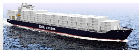
• TOTE Line has ordered 3,100TEU container ships propelled by MAN low-speed ME-GI gas (DF) engine. (Route: Florida⇔ Puerto Rico)
