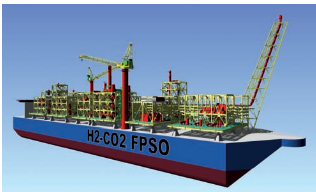
The new H2/CO2 FPSO concept design developed by Mitsubishi Heavy Industries (MHI) and Chiyoda Corporation which received ClassNK approval in principle
