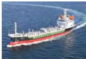
RYOUMEI MARU 749 gt ASPHALT CARRIER built by MIURA SHIPBUILDING CO., LTD. for KYOKUJU SHIPPING CO., LTD.
